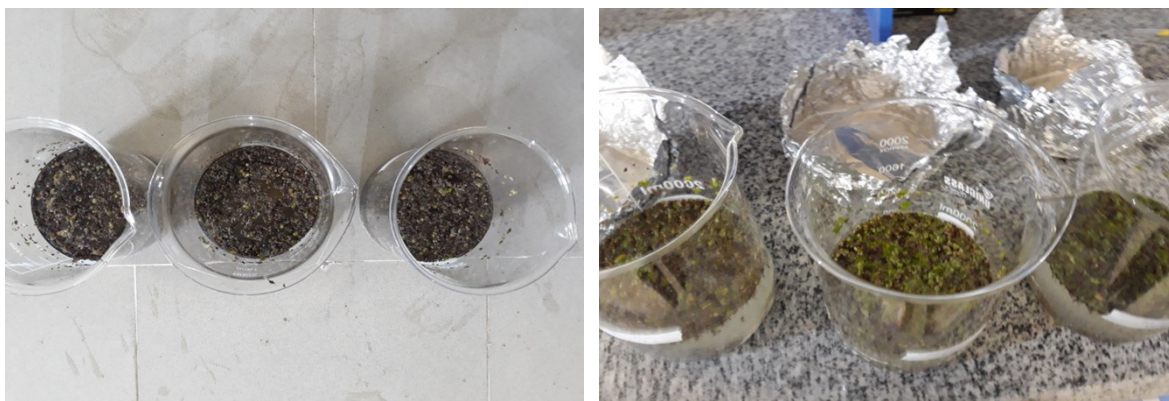
Figure 1. Flasks containing 3.0 grams Azolla and 1000 mgL -1 TPH : first day (left), after 14 days (right)
